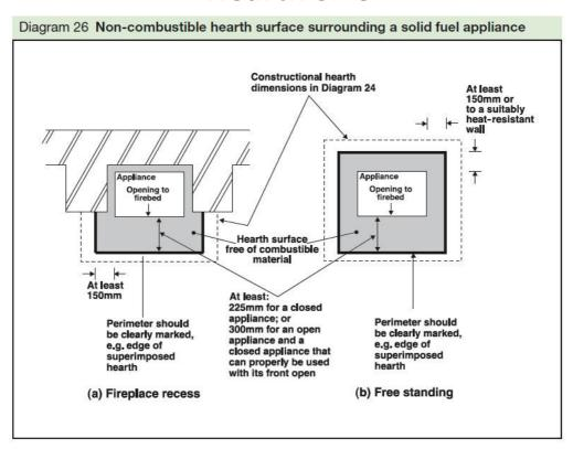
The stove must sit on a hearth of non-combustible material extending a minimum of 150mm (6") out from the stove at the sides and 300mm (12") in front.
